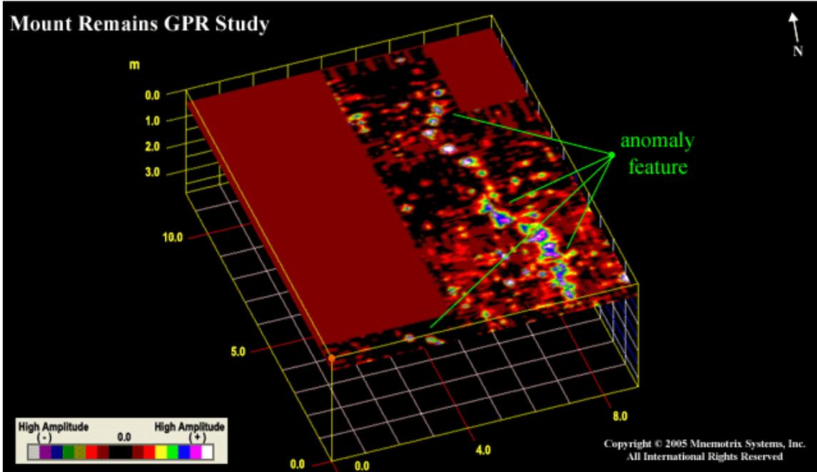
Figure 1: Here you can see a distinct feature running roughly NE through the grid. The slice is located about 0.5 m below the surface.
