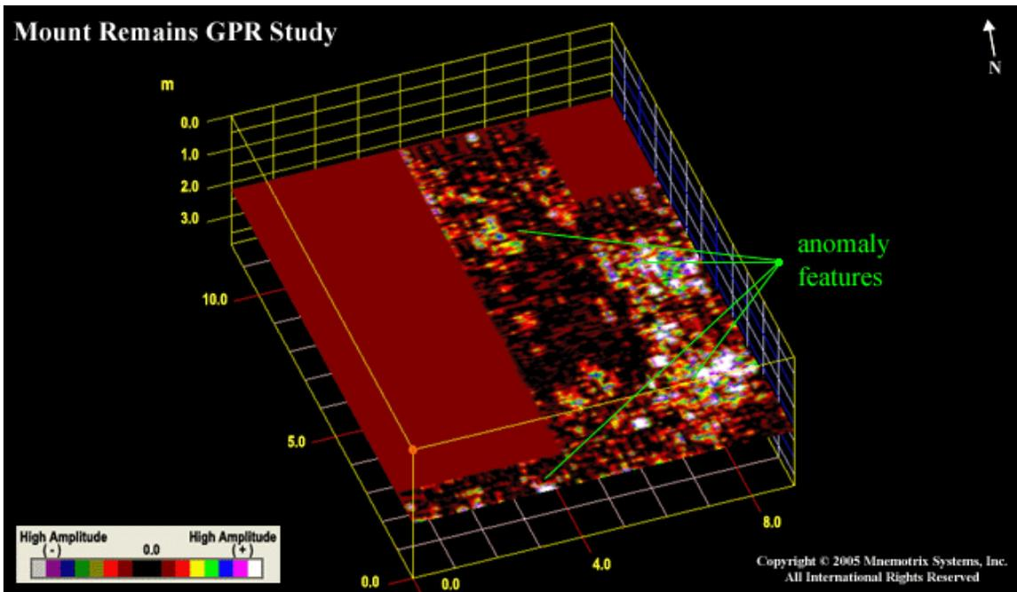
Figure 2: Here 4 areas have been marked as anomalies. The white color indicates a very strong reflection/change in the subsurface between the matrix and the anomaly. We suggest starting work at these areas of white when beginning excavations in this large area. Depth slice is located about 2.2 m below the surface.
