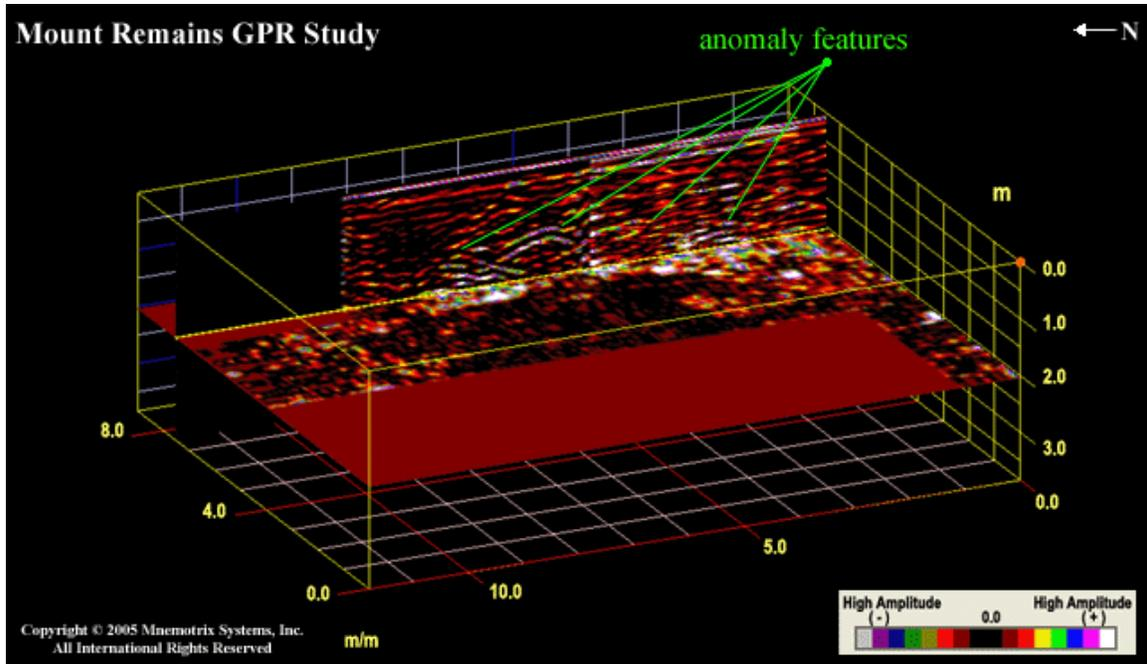
Figure 3: This is a side view (X-axis) of the anomalies from Figure 2 above. What is seen here are the main hyperbolas/reflections that are the apex of the anomalies creating the “white space” in Figures 1 and 2 above. Depth slice is about 2.0 below the surface, while the X-slice is about 1.5 m west of the eastern grid border.
