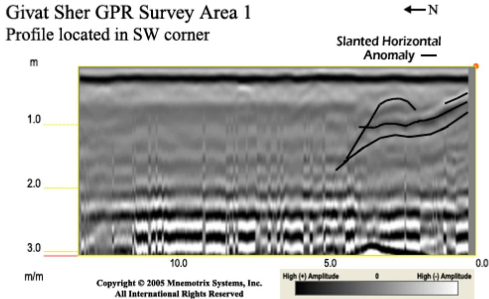
Figure 2: This side-view x-slice is part of GPR Area 1, located in the SW corner of the grid. A slanted horizontal anomaly has been traced (~35 – 45 degree angle), evidenced by the sloping lines and hyperbolic reflection. The anomaly extends about 4 meters N from the southern grid boundary and about 5.5 meters E of the western boundary. This anomaly can also be seen in Figure 3 below as an X.
