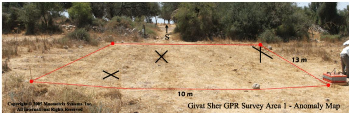
Figure 3: Anomaly map for GPR Survey Area 1. Three anomalies seen in the GPR data were studied and their locations have been marked by an X. The northernmost anomaly begins around 1.7 meter depth, becomes a large/round anomaly at 1.9 m, then stronger at 2.07 m. The feature is about 1 meter wide and stays consistently visible until 3 meter depth. The middle anomaly is similar in size and depth to the northernmost anomaly.
