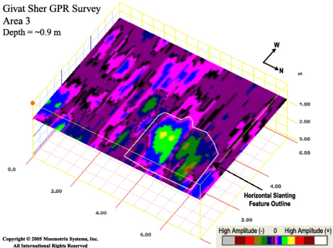
Figure 7: This is a top view of the same reflector from Figure 6 above. The anomaly seems to be quite wide, about 4 meters E/W and 3 meters N/S. In Figure 8, it can be seen that this is a place of depression. Past the southern end of the grid is a cistern, possibly built at a time when the soil height was shallower. It is possible that this anomaly is related to the mentioned cistern. Only ground-truth excavations can solve the true identity, located less than 1 meter below the surface.
