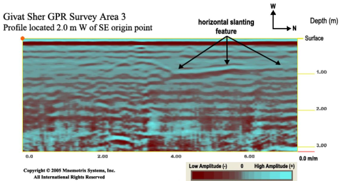
Figure 6: In this figure a horizontal slanting feature is clearly visible. It is seen here in profile view and from the top in Figure 7. This seems to be a most promising reflector due to its consistency and form. Ground-truth excavation of this feature will be particularly interesting to the authors.
