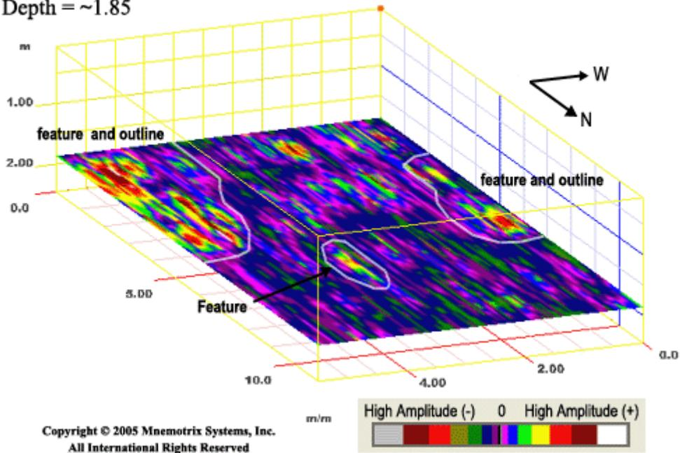
Figure 4: Three main anomalies were visible in the Area 2 GPR survey and are outlined above. The easternmost feature seems to be remnants seen in the sub-surface of the elevation change from excavated trench to ground level, and thus have not been marked in Figure 5 below.
