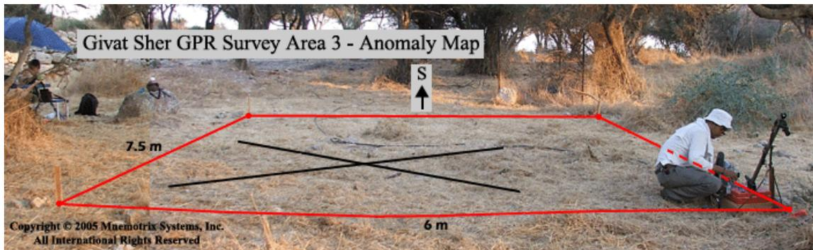
Figure 8: Anomaly map from GPR Survey Area 3. The anomaly discussed in Figure 7 is demarcated as a large X – marks-the-spot.
