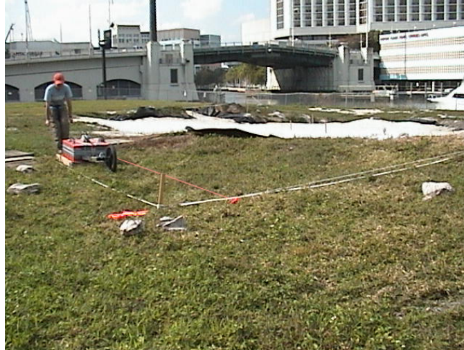
Figure 1: Guideline Cord 200 MHz data acquisition of the Miami Circle (looking NW). Notice the red guideline cord to the left of antenna for maintaining proper distance within the grid while acquiring GPR data.
