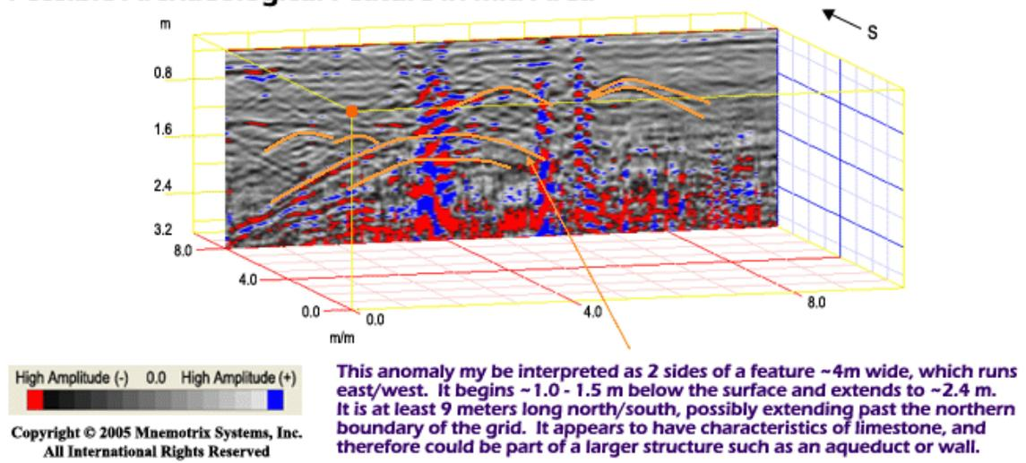
**Figure 7: GPR anomaly in Grid 3 showing possible archaeological feature.**
