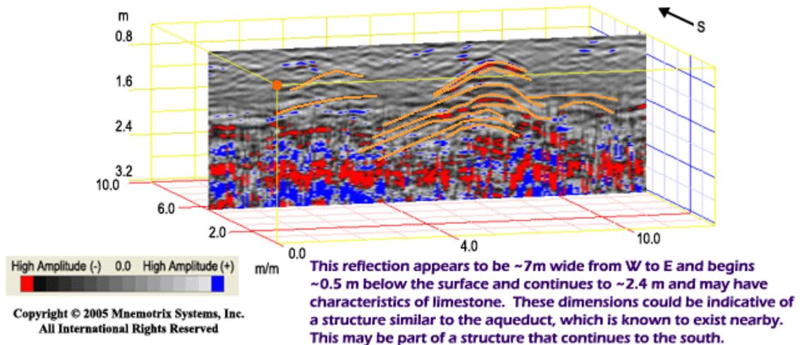
**Figure 5: GPR anomaly in Grid 1 showing possible archaeological feature.**
