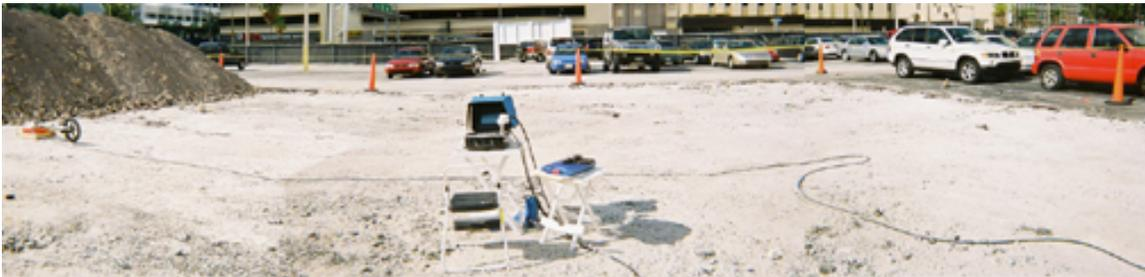
During post-processing, the GPR signal data collected for the southern area was analyzed closely as to depth (vertical axis) and movement along the horizontal axis in a 3D cube.
